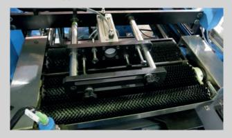
Lug aligner is provided for reliable lug alignment with easy and fast setting features. Vertical alignment of the elements is ensured through vibrating table equipped with efficient pnuematic vibration kit operating without lubrication requirement. Vibration table provided with easy and fast height setting stoppers. Separator alignment is also provided with easy and fast setting stoppers.
