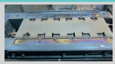
Standard machine is supplied with electric heating pot with 1000 kg capacity. Pot is supplied with thermal insulation and top cover. Machine is supplied with frame integrated suction collection tower for better space utilization.
