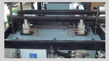
Vertical alignment of the elements is ensured through vibrating table equipped with efficient pnuematic vibration kit operating without lubrication requirement. Vibration table provided with easy and fast height setting stoppers. Separator alignment is also provided with easy and fast setting stoppers.
