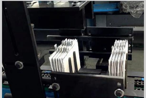
Machine can process most of the plates in automotive size and medium VRLA battery processing.
