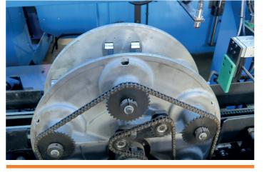
Three row belt vacuum conveyor to transfer the plates from horizontal conveyor to main track. Vacuum seperation & plate release unit to ensure smooth plate drop on to the main track. Toothbelt drive transmission to reduce noise at the main drive.
