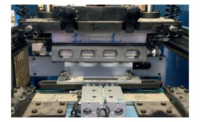
Stainless steel main heat platen with high quality split sheath heaters, which ensures unsurpassed service life. CAD designed and CAM machined aluminum alloy mirrors. Lid holder fitted with lid pickup detection and with unique design pickup mechanism for precision processing. Quick couplers for compressed air and electric connection provided for lid holders. Pneumatic lid holder fitting system for easy and fast changeover.
