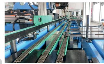
Three axis servo driven weld head with pnuematic compensator for Z axis drive. Chain driven conveyor with battery lifting unit at the welding station. Quick and easy setup battery fixing mechanism. Machine is available to process wide range of 1x6 and 2x3 cell batteries available in the market.
