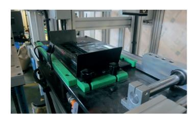
Battery lids are handled by means two independent servo driven pick and place units. Each units has its own parameters configured through HMI.
