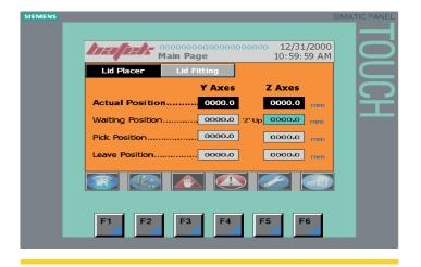
Siemens operator interface in English providing recipe building, motion control settings, manual buttons, diagnostic, alarm definitions, production figures.
