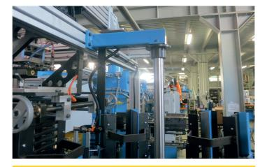
Rotary lid storage magazine has 6 lid storage units all of which can be centrally adjusted in width and length. This facilitates battery type changeover. The machine automatically switches lid storage units Lids are automatically feeded for pick and place unit by lid elevator integrated into the feeding magazine.
