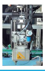
The machine is supplied with an alphanumeric dot matrix code marking unit. The unit can be provided for top or side marking. Easy and quick setup features are integrated in the unit.
