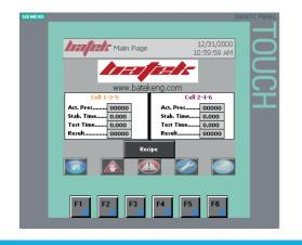
HMI for user friendly operation. Settings, manual buttons, basic production figures, recipe building, alarm & diagnostic are provided at HMI.
