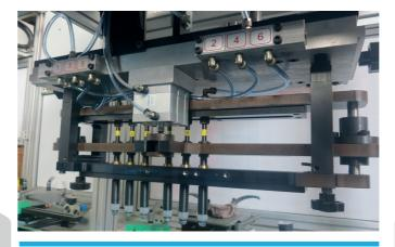
Dedicated tests available for particular lid designs. Kamina test head design mechanically blows all testing seals to tightly seal horizontal vent holes. Easy and quick fit testing head design remarkably facilitates changeover procedure.
