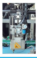
The machine can be supplied with an alphanumeric dot matrix code marking unit. The unit can be provided for top or side marking. Easy and quick setup features are integrated in the unit.
