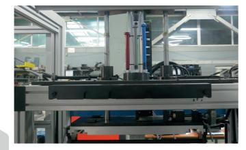
Easy and quick height setting through dedicated stoppers and quick changeover templates for each lid type provided. Additionally fine tuning setting is provided to compensate variations in lid models. Typical changeover time is less than five minutes for complete machine.
