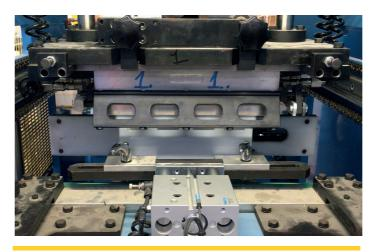
Stainless steel main heat platen with high quality split sheath heaters, which ensures unsurpassed service life. CAD designed and CAM machined aluminum alloy mirrors. Lid holder fitted with lid pickup detection and with unique design pickup mechanism for precision processing. Quick couplers for compressed air and electric connection provided for lid holders. Pneumatic lid holder fitting system for easy and fast changeover.
